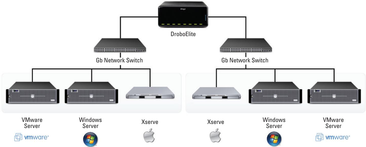
The illustration above shows a sample deployment of DroboElite being used for consolidated storage in a mixed environment featuring both virtualized and non-virtualized host computers.
